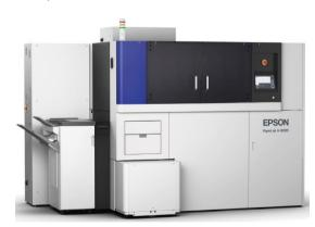
PaperLab not only allows you to close the paper cycle on site but also consumes less water and energy compared to industrially produced fresh fibre or recycled paper. The production of 500
